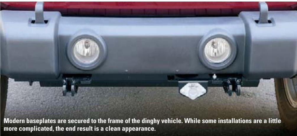
Modern baseplates are secured to the frame of the dinghy vehicle. While some installations are a little more complicated, the end result is a clean appearance.
