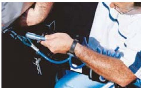
**Plug receptacles added to the dinghy and coach allow easy hookup of an electrical connector for taillights, turn signals and the supplemental braking system.**
