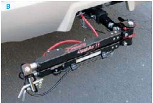
**A)** Once the tow bar is pinned in the hitch receiver, make sure electric connections and safety cables are secure. **B)** While driving your dinghy, this type of tow bar remains on the coach, tucked out of harm's way.
